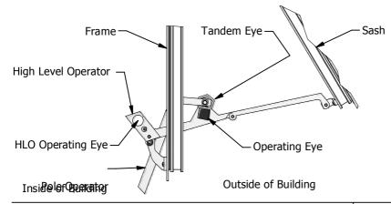
Attempt to close the window with a pole operator. At this stage the tandem eye and operating eye are often out of sight to the operator. This is becasue they have moved over outside of the window.
